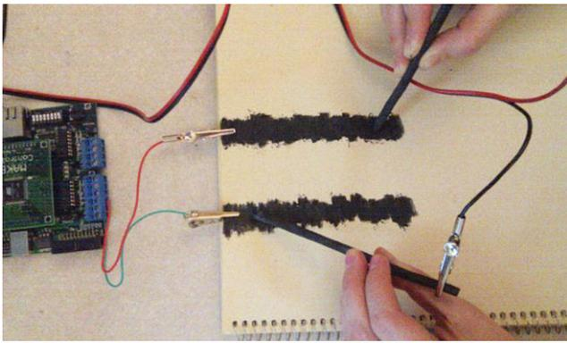
**Fig. 4** Our tangible drawing interface is shown in this figure. On the sheet of paper two regions of graphite have been drawn. These are hooked up to the analog input ports on the Make Controller shown here. Hooked to the positive voltage terminal are two artists charcoals which complete the resistive sensing circuit
