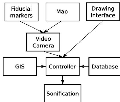
**Fig. 2** A flowchart of the system organization of our system. This system has at its core a Controller module that communicates with the phenology and GIS databases as well as the video camera and sonification engine. It generates sonifications by tracking the positions of fiducials on a printed paper map
