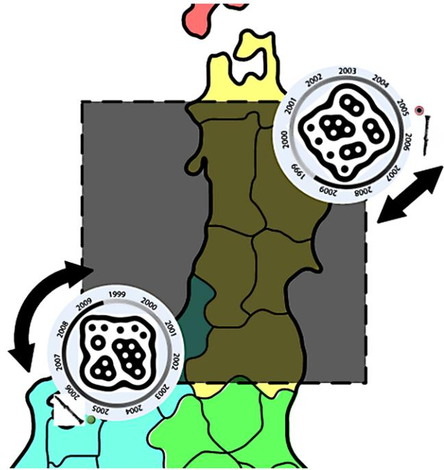
**Fig. 5** Moving a fiducial will sonify data that is represented by map locations under that particular fiducial marker. These fiducial markers and the map itself are printed out on heavy stock paper in an ordinary printer
